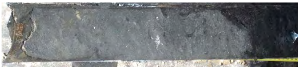
Photo 7. Vibrocore VC5C(0.0-0.5m) from Dredge Area 3 showing silty sand overlying clay.
