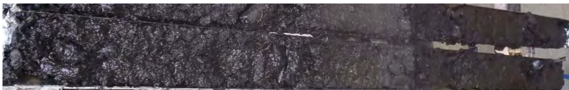
Photo 6. Vibrocore VC5E(0.0-1.65m) from Dredge Area 3 showing broken up peat/mud overlying clay.
