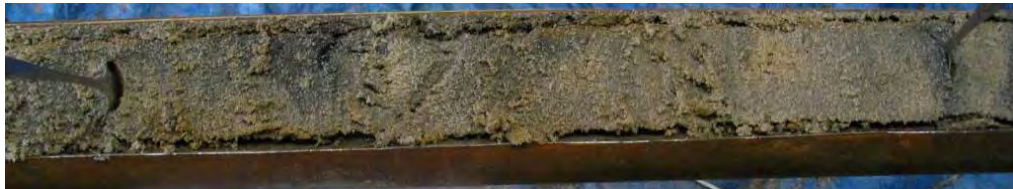
Photo 4. Vibrocore VC4B(0.5-1.0m) from Dredge Area 1 (Swing Basin) showing silty sand.
