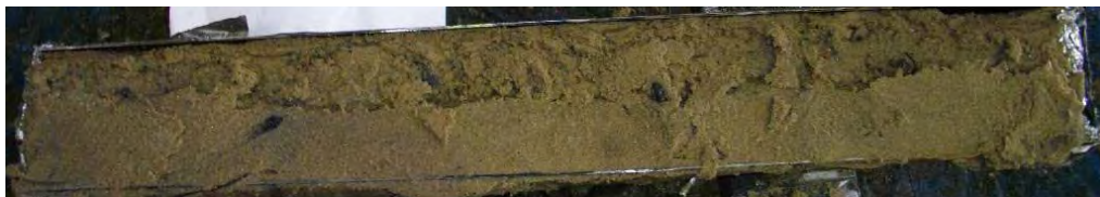
Photo 5. Surface core SS4A (0.5 m to 1.0 m depth) from Dredge Area 1 showing sand.
