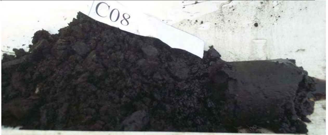
Plate 3. Consolidated very hard and stiff dark brown to black organic-rich flaky peat (dry in situ ) (47% fine fraction and 19% TOC content) from the eastern part of the Berth 1 Dredge Area Sample location C8).
