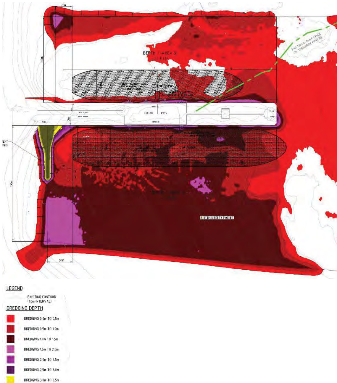
Figure 2. Areas and depths of proposed dredging in Dredge Area 3 (Berths 1 and 2). Note the widening of the proposed dredge area in the lower right of Berth 1 (i.e. the northeastern margin of Berth 1) relative to the dredge footprint shown in the Supplementary SAP (Appendix 2).
