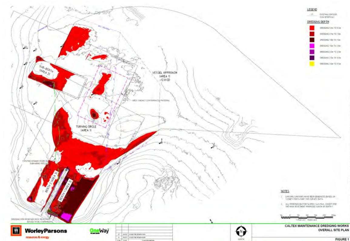
**Figure 1.2 Overall site plan, showing proposed dredging works. (Source: WorleyParsons)**
