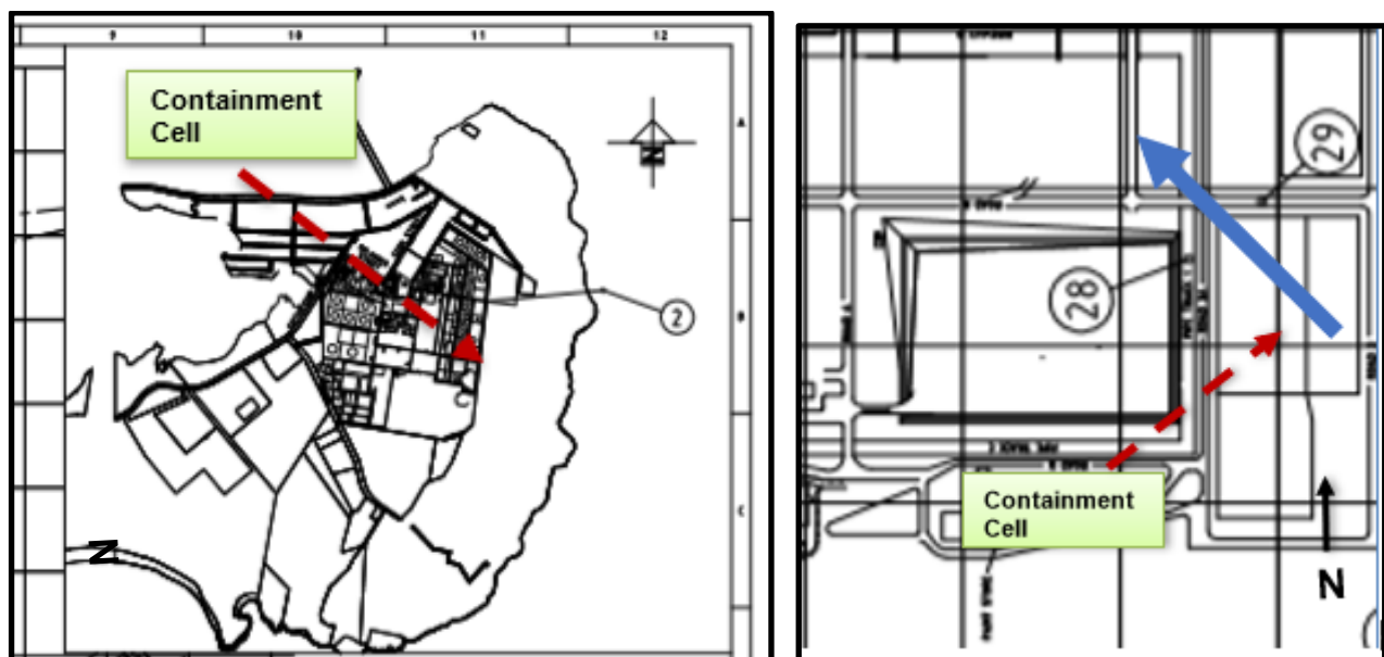
Figure 5 Schematic Location Plans for Monitoring Wells EPL28 (28) and EPL29 (29). The left side shows the whole Kurnell site and the right side is zoomed in to the Containment Cell with the two monitoring wells on the north-west (28) and north (29). The blue arrow is the general direction of groundwater flow at the Containment Cell.
